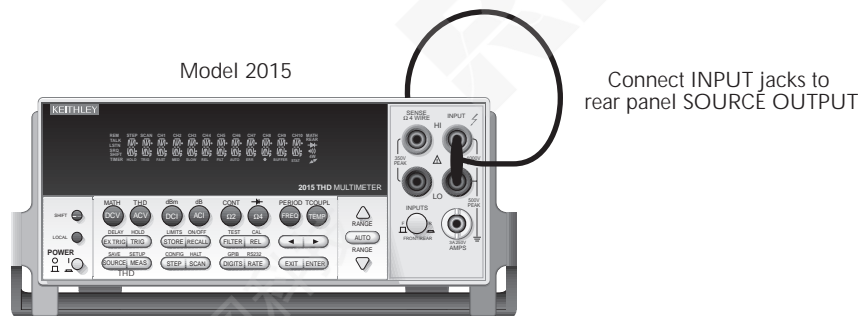
Figure 2-6 Connections for function generator calibration
