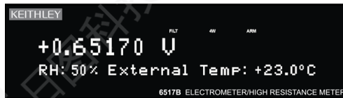
Figure 43: Relative humidity and external temperature display
