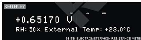
Figure 7: Relative humidity and external temperature display
