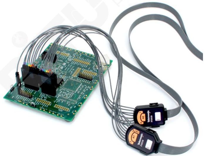
P5910 17-channel general purpose probe
