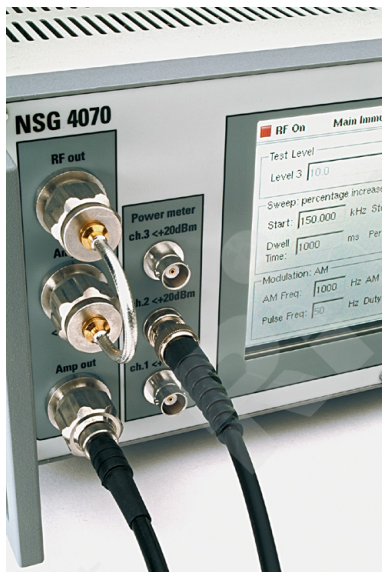
NSG 4070 front panel with RF ports
