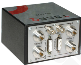
SW 4070, RF switch network 2xSPDT
